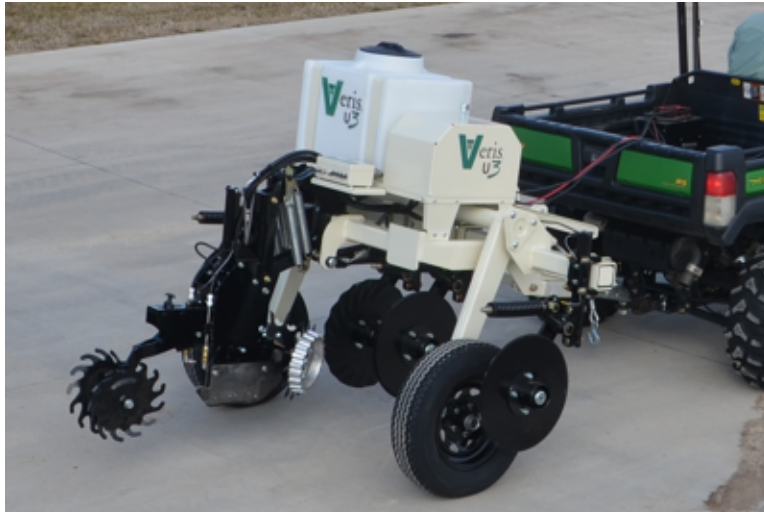
Figure 5. Veris U3 system with EC, Vis-NIR, and pH sensing.
