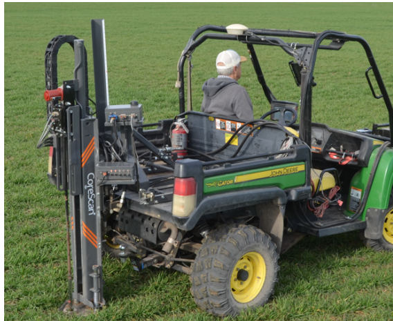
Figure 2. Veris CoreScan platform--UTV mounting. Figure 3. CoreScan sensing technologies.
