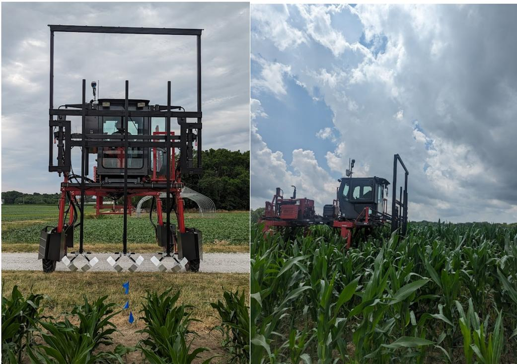
Figure 1. The OATSMobile system. Based on a 2016 Lee-Agra sprayer, equipped with multiple communications devices and sensor systems for enabling communications with in-field sensors and other computing assets in rural environments.
