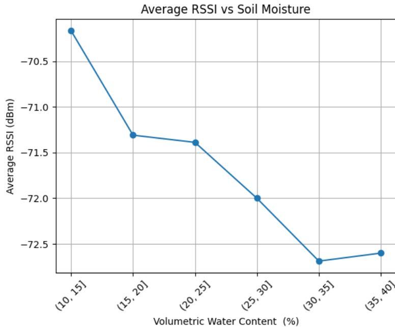
Figure 8. Average RSSI for different levels of volumetric water content in soil.
