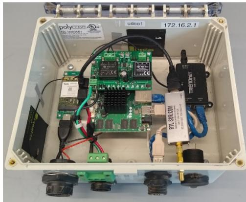
Figure 2. The ISOBlue edge-computing device. A network-based architecture allows to extend the functionalities in a modular approach.
