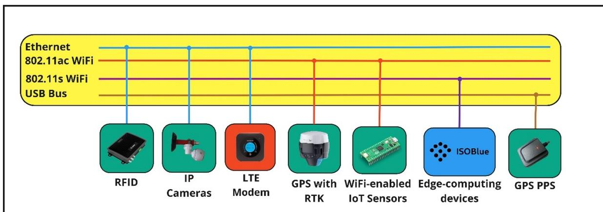
Figure 3. Communications with data sources in the OATSMobile system. By featuring multiple networks and data buses (yellow), OATSMobile can communicate with a variety of sensors (green), other edge-computers in a fleet (blue), and network backhaul devices (red), such as LTE modems for access to commercial backhaul networks.
