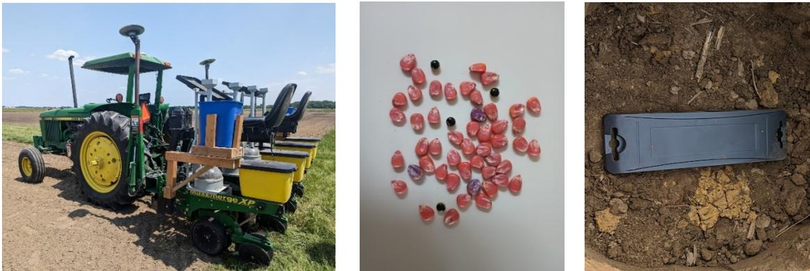
**Figure 5. Research plot planter used to plant the small tag units (left). Small RFID tags compared to regular corn seeds (center), and a large RFID tag featuring a weatherproof enclosure, for deep underground communications testing (right).**
