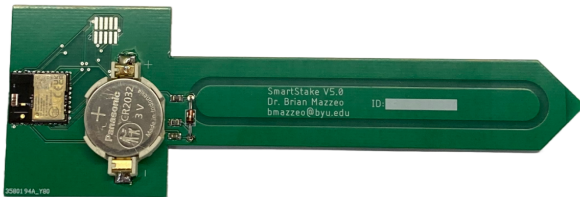
Fig. 2 Smart Stake before weatherproofing.
