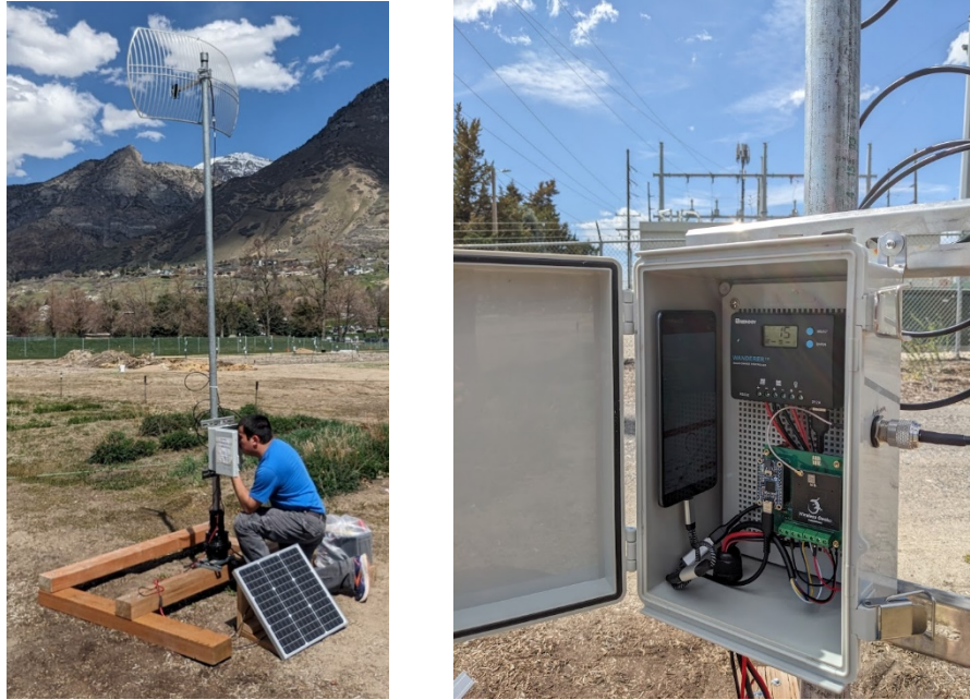
Fig. 3 (Left) Receiver with mast and high-gain antenna deployed at BYU Life Sciences Greenhouse plot. (Right) Receiver junction box internal electronics, including solar charge controller, mobile phone, and BLE receiver SoC.
