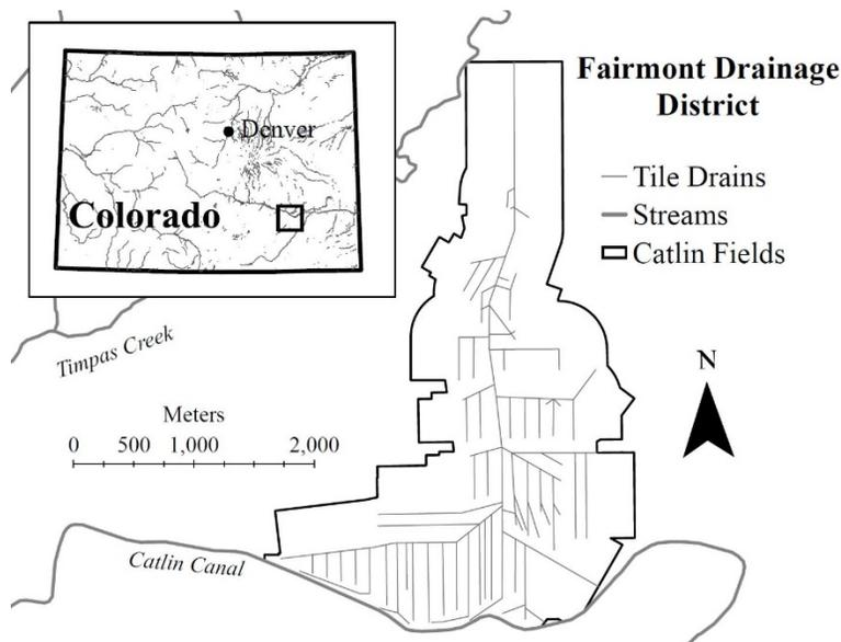
Fig 1. The FDD in the LARV with the layout of the tile drains.
