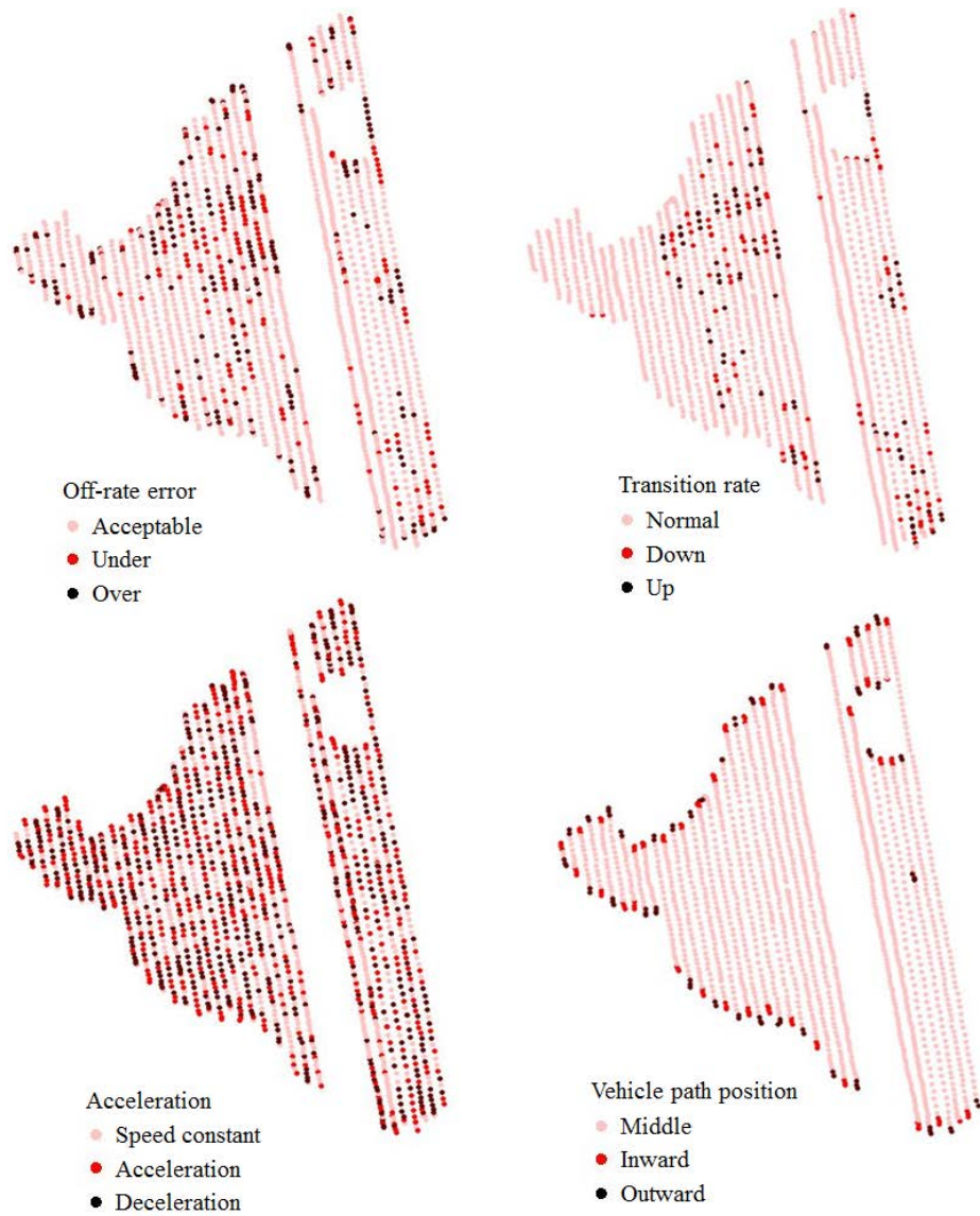
Fig. 3. Maps of off-rate error and possible error sources classification on a corn field fertilization.
