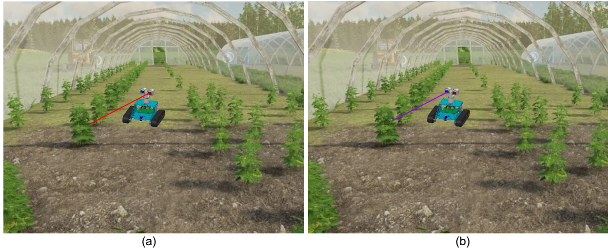
Figure 1. A Simulation for the proposed weed detection and control system, (a) on the left side shows a simulation for the robot in a greenhouse during the detection process using the laser speckle imaging technique, while the image in the right (b) illustrates the control process by a UV-C LED
