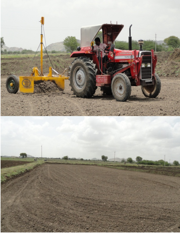
Fig.1.Operational View of Laser leveler and view of laser leveled field
