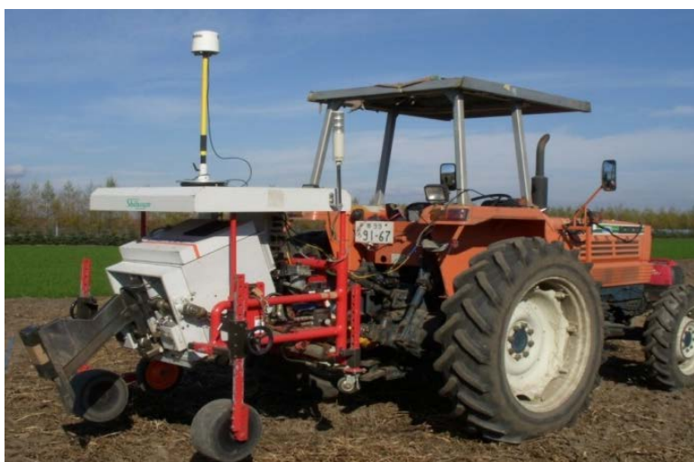
Figure 2. Real-time soil sensor (RTSS) used in the experiment.
