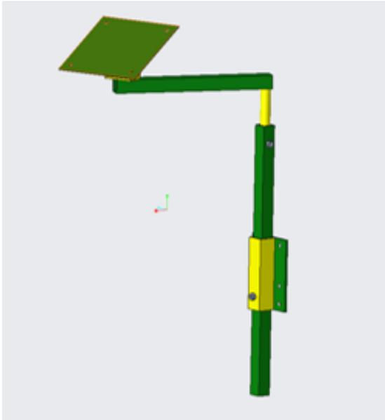
Figure 2.5 The bracket mounted on the implement
