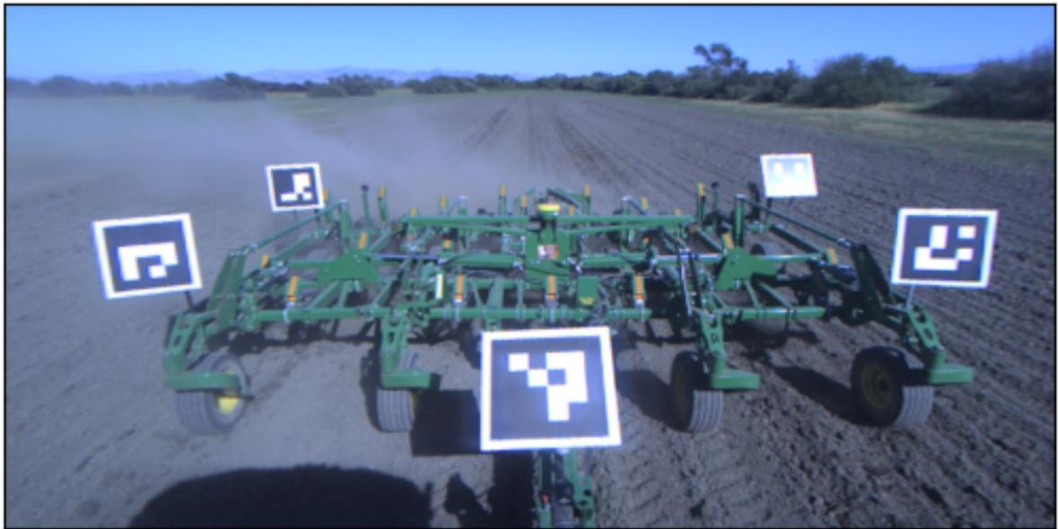
The ArUco markers are correlated together in an image, and the script will identify the markers as the ‘corners’ of the implement. Then, the corners will utilize the stereodepth metadata associated with the pixels to identify the point locations in 3-dimensions. Finally, these points will be utilized in the robotics pipeline to identify the position of the implement in 3-dimensions. The remainder of the robotics stack will utilize the newly identified implement position for downstream tasks.
