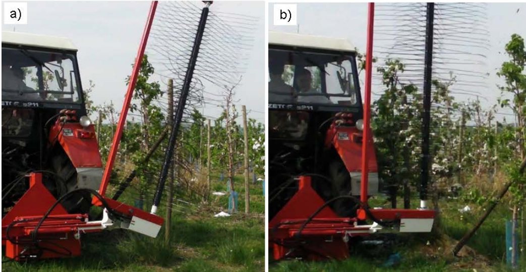
Fig. 6. Adaptive mechanical thinning unit; a) tilted and b) upright position
