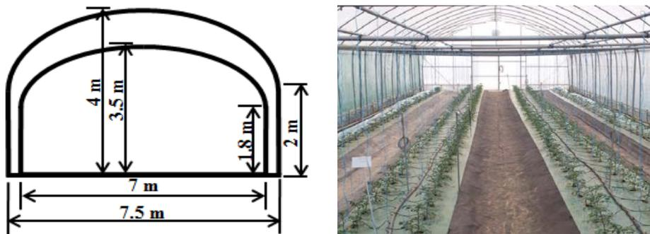
**Figure 2.** Dimensions (left) and view (right) of the cherry tomato-growing greenhouse.
