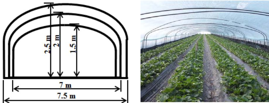
**Figure 1.** Dimensions (left) and view (right) of the strawberry-growing greenhouse.
