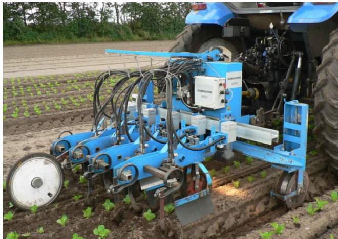
Fig. 1. Picture of the Robovator performing mechanical weeding in transplanted lettuce. Source: visionweeding.com
