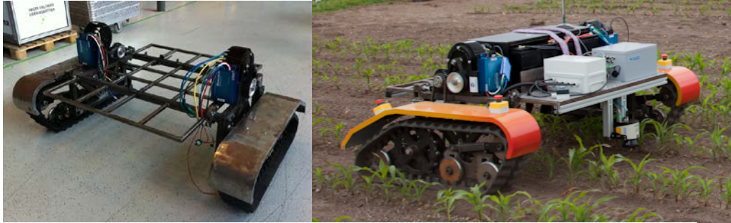
Fig. 2. Left: The Armadillo frame, tracks, and motors assembled. Right: The Armadillo driving in a maize field.
