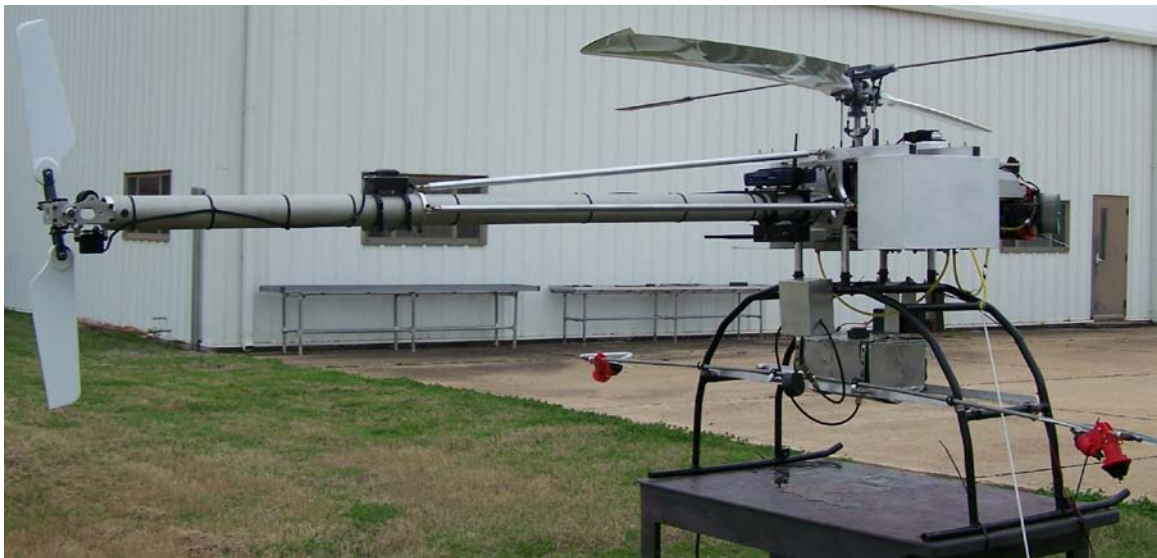
Fig. 1. SR200 UAV helicopter spray system with spray system mounted on the undercarriage.
