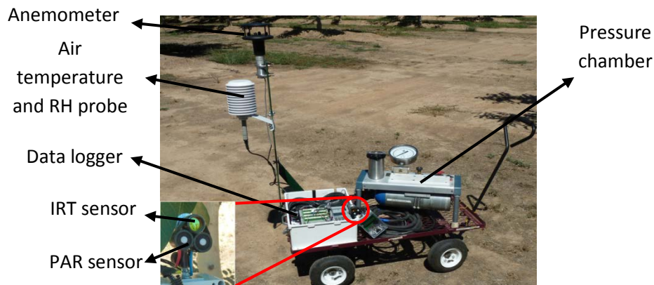
Fig.1. Mobile sensor suite and pressure chamber during data collection in an almond orchard.
