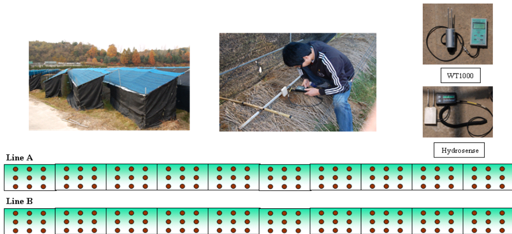
Figure 1. Measurement of soil water content variability using 2 commercial sensors at different locations and depths.
