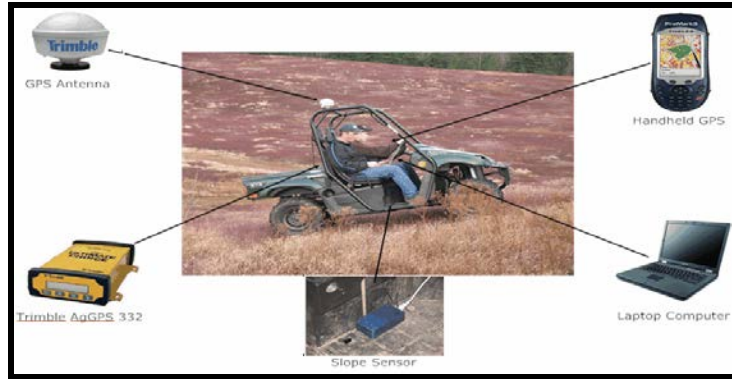
Fig. 1. Slope Measuring and Mapping System (Zaman et al., 2010).
