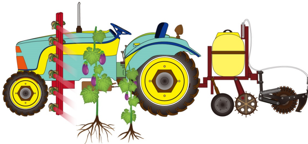
Figure 2. Structural diagram of variable rate system for soil disinfection showed six sensors fixed to both front sides of the tractor to detect target crops.
