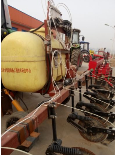
Fig. 8. Soil variable injection system included disc, plow and injector, and traveled by traction in the field. The outline of the soil variable injection system could be figured out.
