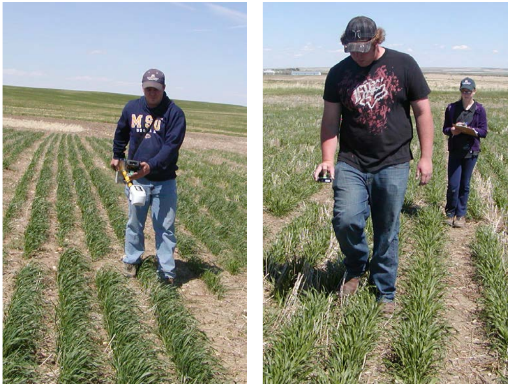
Figure 1. R. Christiaens, Research Associate, and J. Jerome, Research Assistant, obtaining spring wheat reflectance measurements using GreenSeeker Sensor (left) and Pocket Sensor (right), Conrad, MT, Spring 2012.
