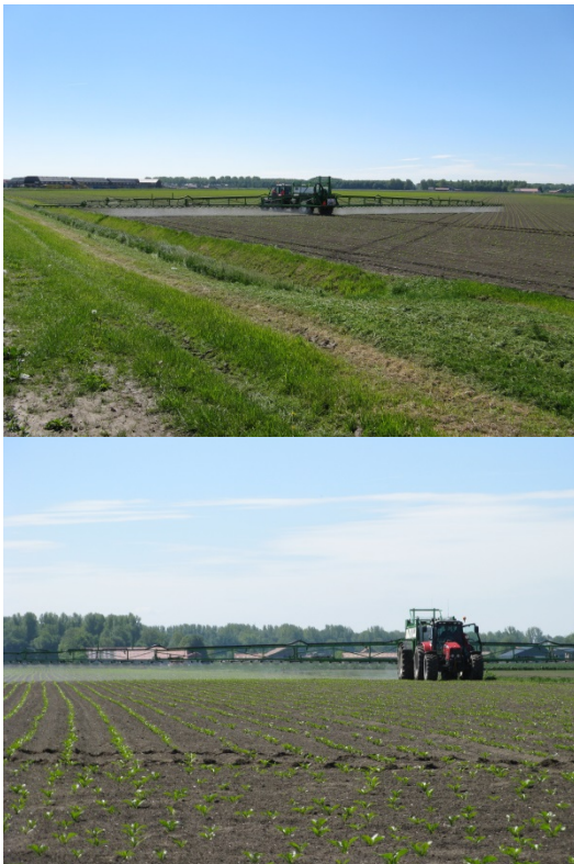
Figure 2. Overview of field test with VRA task map spraying in sugar beet.
