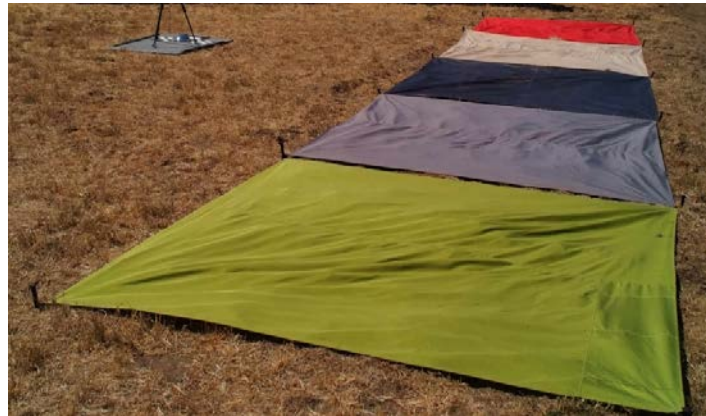
Fig. 3. Calibration tarps were set out for each flight. Tarps were 2.8 m by 2.8 m.
