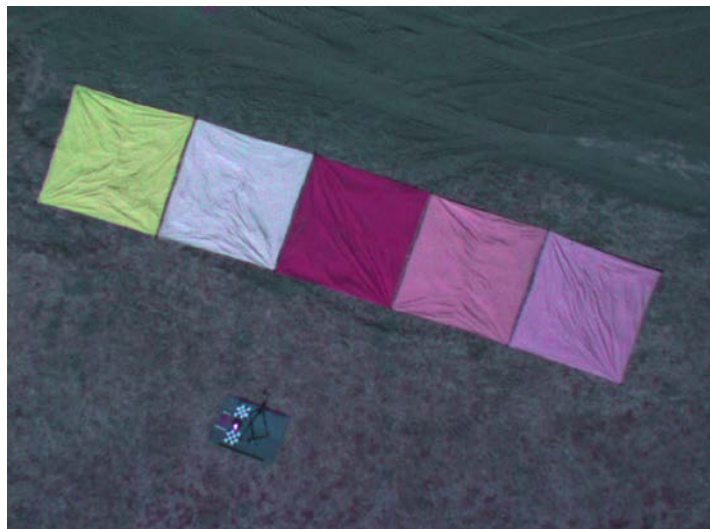
Fig. 5. Color-infrared image of the calibration tarps acquired on June 22, 2013. From left to right, the tarps are red, beige, dark blue, gray, and light green (see Fig. 3). Pixel sizes varied between 1 and 4 cm, depending on altitude and view angle. In this image, pixel size was 1.2 cm.
