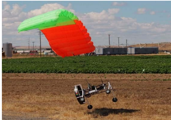
Fig. 2. A Tetracam small Unmanned Aircraft System (sUAS) is shown taking off with a Tetracam Agricultural Digital Camera Lite for acquisition of near-infrared (NIR), red, and green images.
