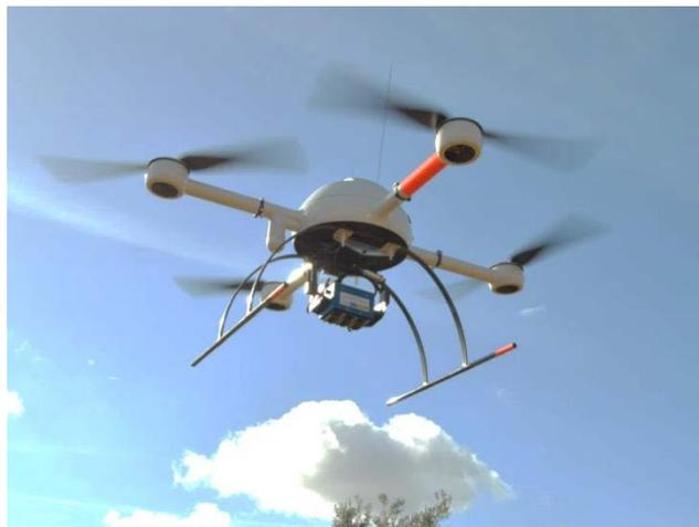
**Figure 1.** Quadcopter platform with the multispectral camera embedded under its belly.
