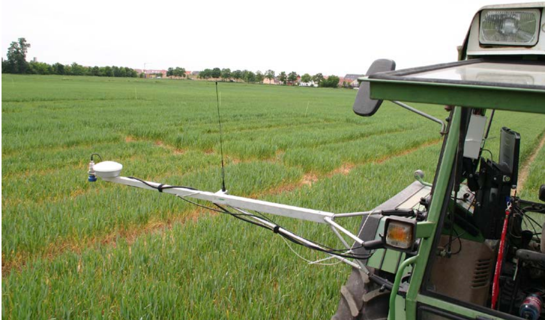
Fig. 2. Test prototype of the ultrasonic sensor (Agri Con)
