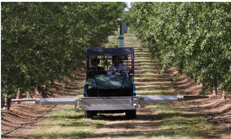
Fig. 1. Lightbar system mounted on a Kawasaki mule.
