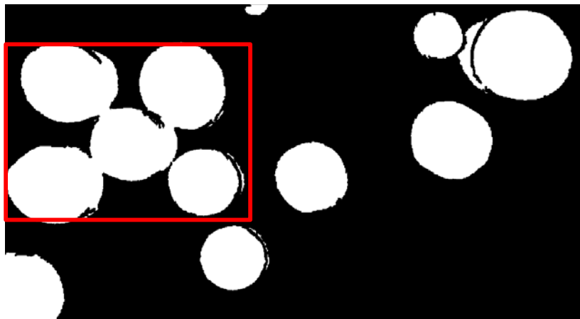
Fig. 5. A result image after thresholding to remove background pixels and filling holes within objects.
