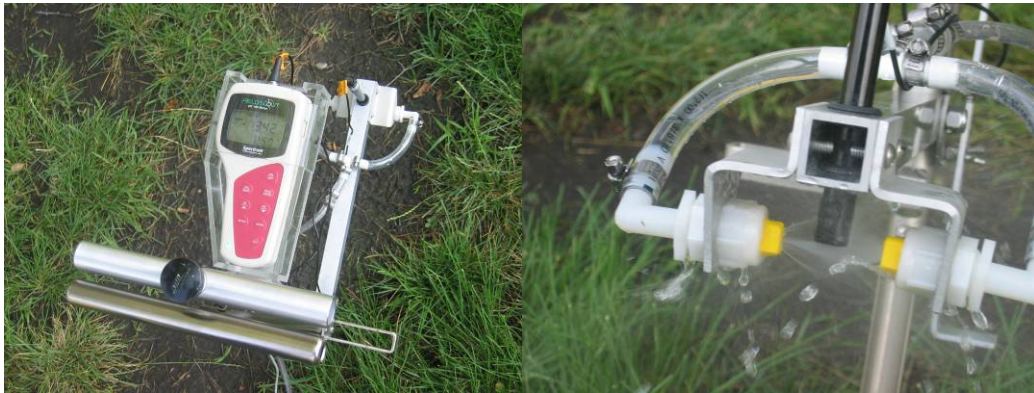
Figure 2. Manual probe for on-the-spot soil ion activity measurements.
