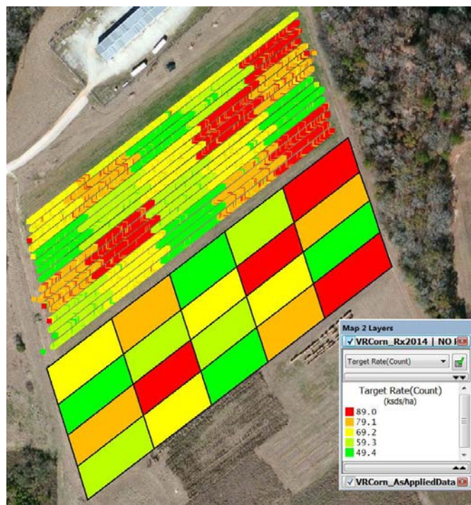
Fig. 3. Side-by-side comparison between the prescription (Rx) map versus the actual as-planted map based on the population information collected using the Biosystems data acquisition system. All maps created using AgLeader SMS Advanced software with units in 1000 seeds ha -1 . Note that the northern most pass was not included in the analysis since it represents a uniform rate.
