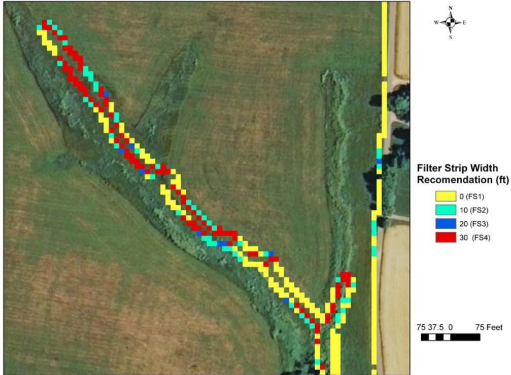
Fig. 2. Map indicating the width of filter strips required to stop 95% of sediment loading for the northeastern region of the field. The class descriptions can be found in the caption of Fig. 1.
