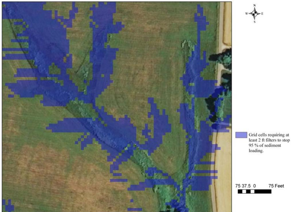
Fig. 3. Map indicating the locations of grid cell requiring at least 2-ft buffers to stop 95% of sediment loading.
