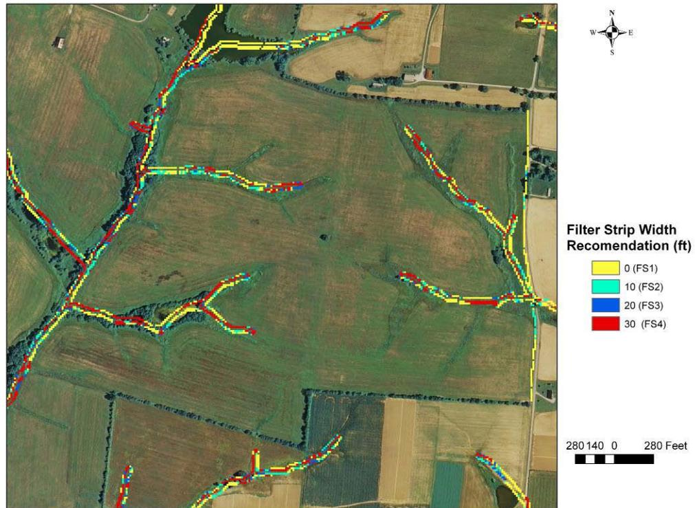
Fig. 1. Filter strips widths required to stop 95% of sediment loading in the northeastern region of the field. The filter strip classes were defined in a way that would make them easy to use by conservation planners in the field. The specific ranges for these categories are given in US feet:  $0 \leq \text{FS1} \leq 5$ ,  $5 < \text{FS2} \leq 15$ ,  $15 < \text{FS3} \leq 25$ ,  $\text{FS4} > 25$ .
