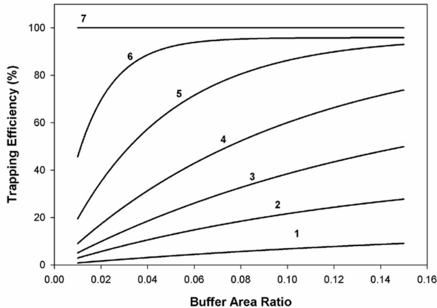
**Fig 1.** Relationships between pollutant trapping efficiency and buffer area ratio for seven different site conditions. The specific conditions represented by each line are listed in Table 1.
