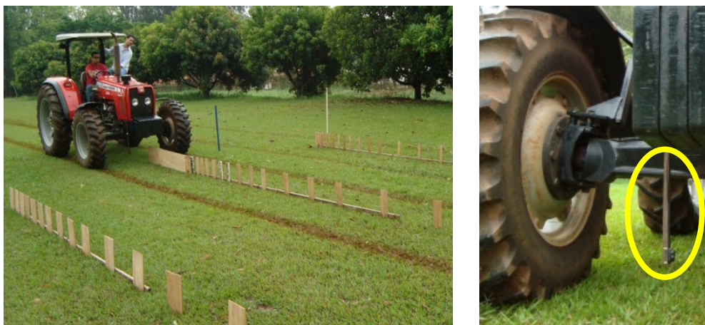
Fig. 1. Test using regular obstacles simulating stalks (left) and photoelectric sensor positioned underneath in front of the tractor (right)
