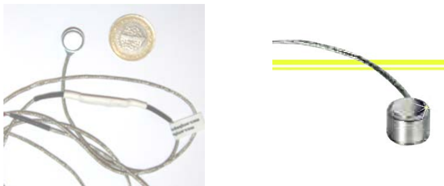
Fig 4- Load cell for force measurement
