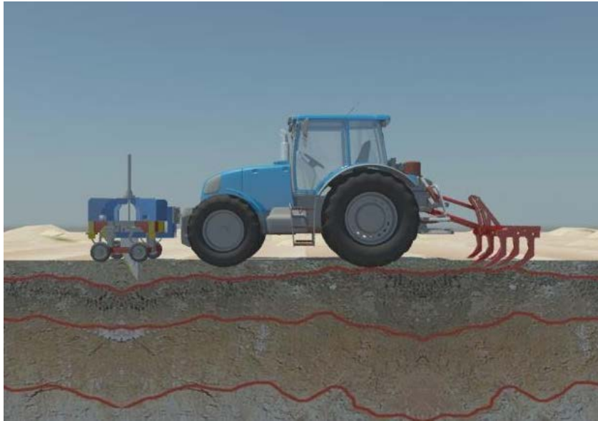
Fig 6- Assembled structure of the Soil Strength Sensor and Chisel on a Tractor
