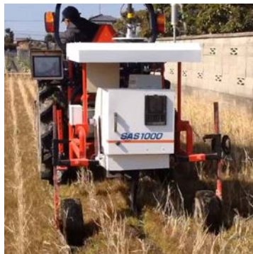
Fig. 2. Real-time Soil Sensor SAS1000
