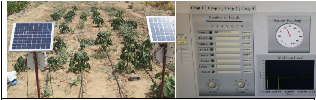
(a) (b) Figure 2.1: (a) Sensor based irrigation control system under preliminary testing; (b) Front-end window of the sensor-based irrigation control system with optional settings
