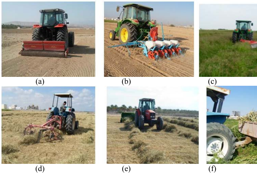
Figure 2.1. Machinery used in the field for different farm activities; (a) Land preparation; (b) Grain seeder; (c) Mower; (d) Rake; (e) Baler; (f) Trailer for transportation (Jayasuriya, et al., 2013).
