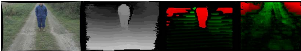
Figure 3. from left to right: 1. Reference HDR image. 2. Depth map from dynamic programming. 3. Plane fit and rotated to ground plane to show height from ground and colour coded for red obstacles. 4. Height from ground without the person, based on SMW subpixel correlation depth map.
