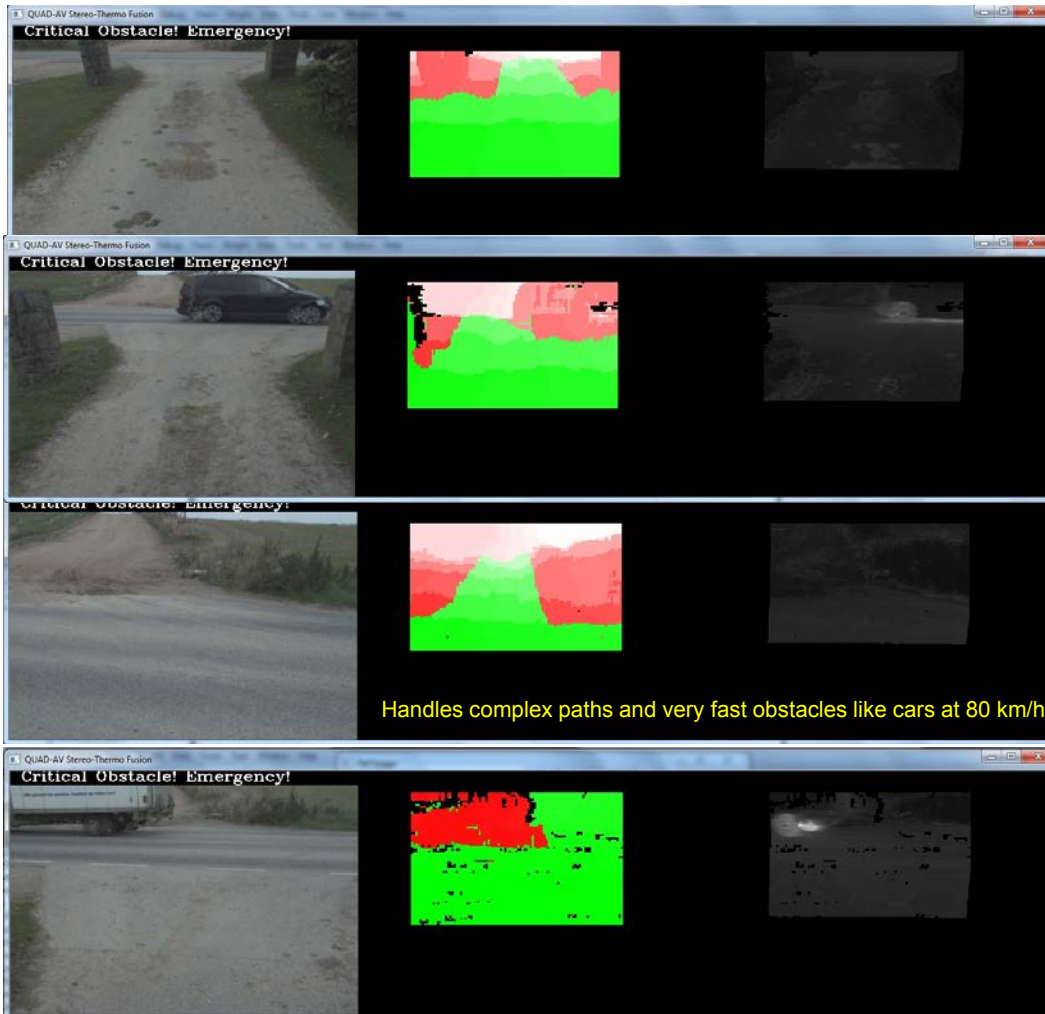
Figure 7. Results shown in the following way: RGB Image / Classified Cells / Thermal Image that has a smaller FOV that limited amount of annotated cells. Green cells: Traversable. Red: Not traversable. Purple/Cyan: Selected cell for showing the GMM classes (when applicable).
