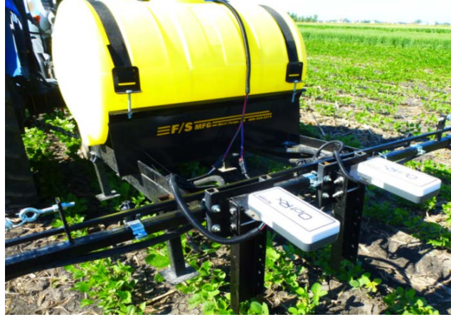
Figure 2. Ag leader OptRx sensors mounted on a tractor.
