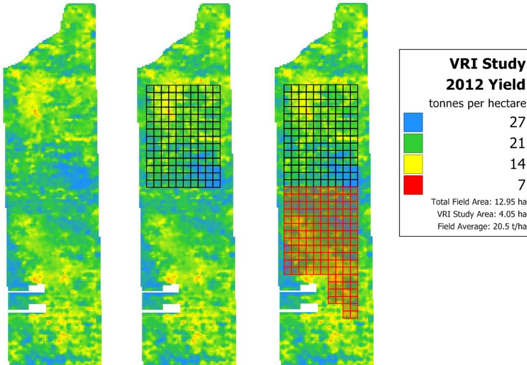
**Fig. 1.** Layout of the variable rate irrigation study (black grid) and an equal area on CI (red grid) for comparison of data. There are 140 (15 x 15 m) zones in each grid. The background vineyard fill is the 2012 yield map.
