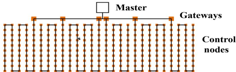
**Fig. 2.** Communication network section representing the master, six gateways and 270 control nodes in 27 vineyard rows. There are either 40 or 50 nodes, corresponding to 4 or 5 rows, attached to each gateway and connected with 800 to 1000 meters of continuous cable in a serpentine pattern.
