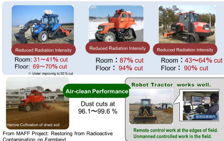
Figure 4. Protected cabins robot tractor against radioactive contaminations.
