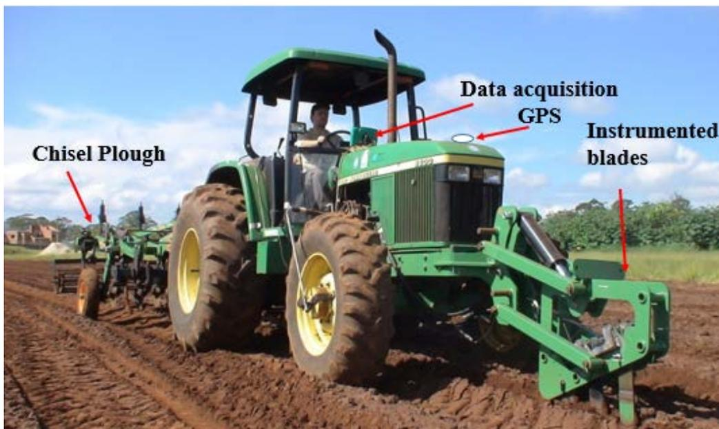
**Figure 1.** Prototype of variable-depth control system composed of system reading of shear strength of soil, GPS, data acquisition and chisel plough
