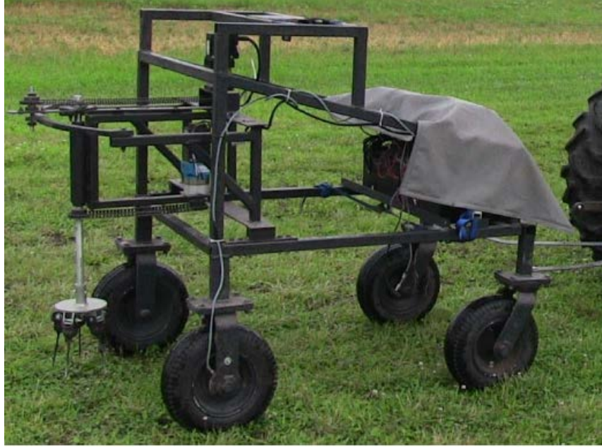
Figure 1: Prototype mechanical weed control system developed at Iowa State University (Ahmad 2012).
