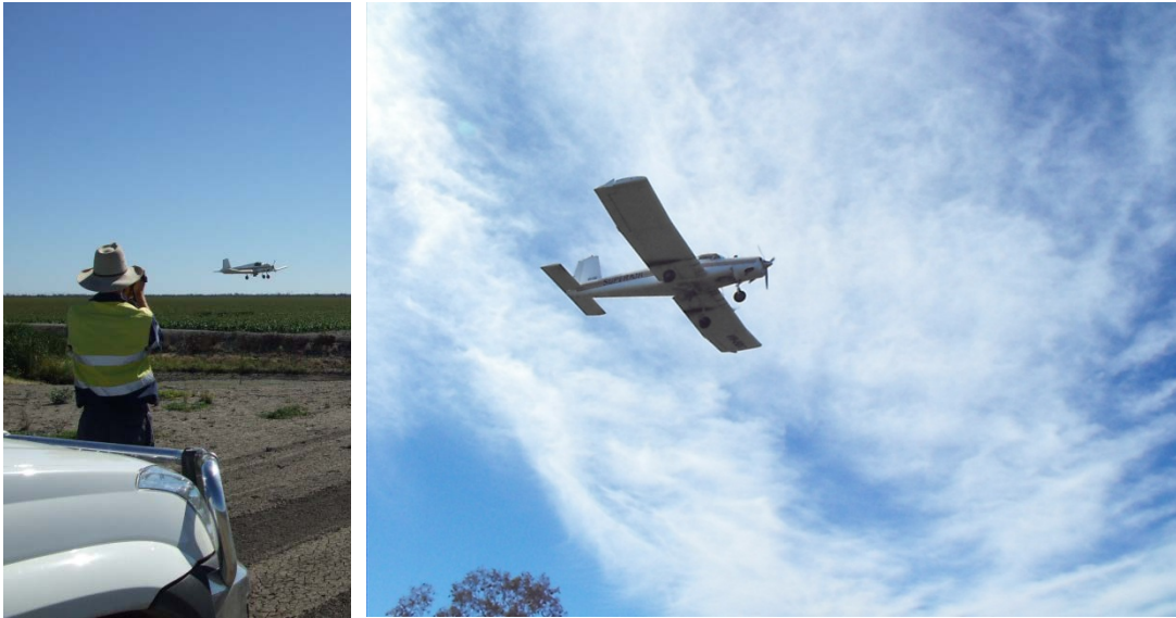
Figure 1. Low-level airborne data acquisition trials using (a) Crop Circle™ ACS-210 at 4 m AGL over a field of sorghum and (b) Raptor™ ACS-225LR at 50 m AGL over a field of wheat.
