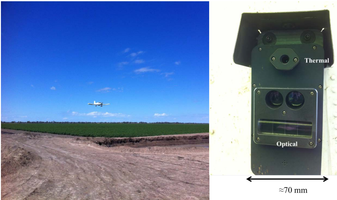
Figure 5. (a) Low-level airborne data acquisition trials using the Raptor TM ACS-225LR-IRT at 50 m AGL over a field of cotton. (b) Close-up view of the Raptor TM ACS-225LR-IRT.
