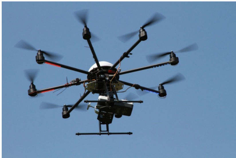
Figure 3. A RapidSCAN CS-45U deployed on an Octocopter. Sensing range is 0.5 m to 4+ meters above canopy.
