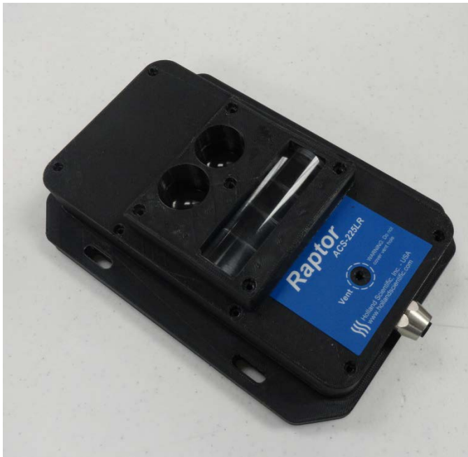
Figure 4. A 3D printed prototype ACS-225LR-U UAV-ready AOS sensor.
