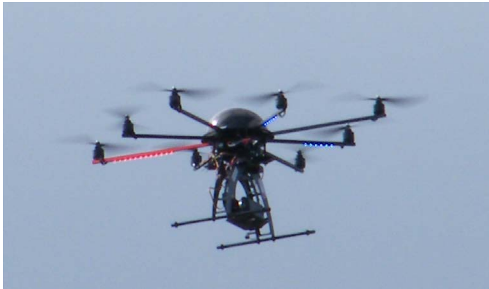
Fig. 2. Octocopter-XL carrying a modified Canon Powershot SX230 HS camera for multispectral imaging.
