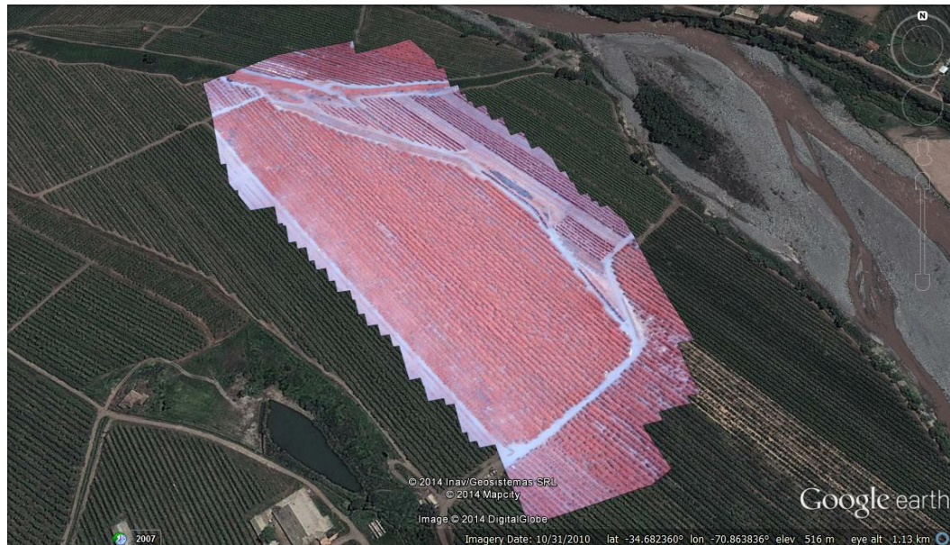
Fig. 5. Orthomosaic of 6 ha sweet cherry orchard using Photoscan Pro to process images geotagged with the UAV GPS. No GCPs were used. See Table 1 for settings.
