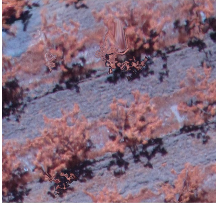
Fig. 7. Artefacts (swirling and smearing effects) sometimes present in high-resolution orthomosaics of trees.
