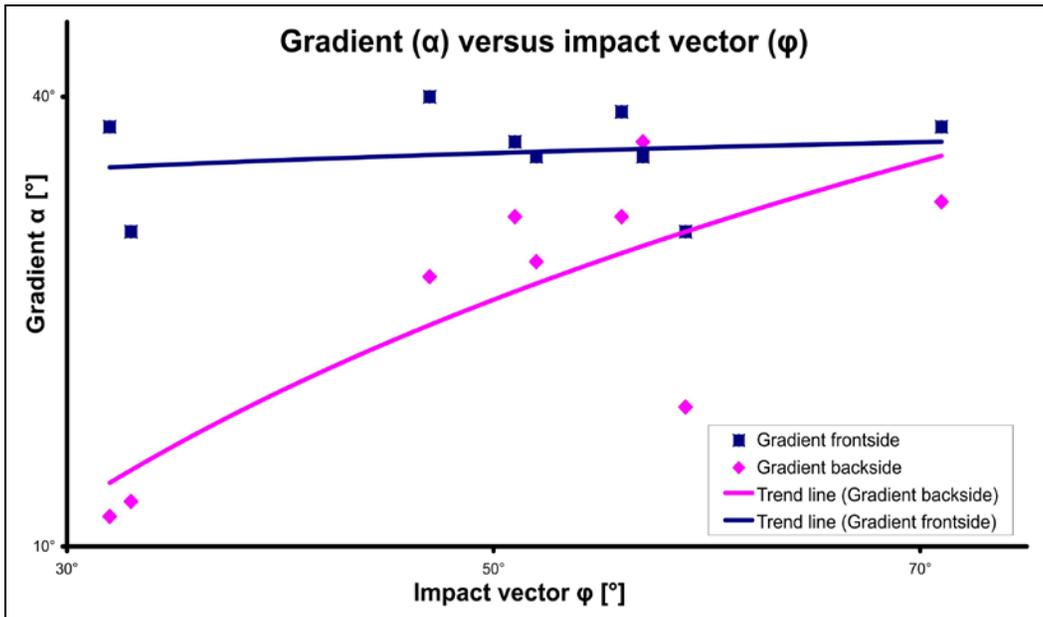
Figure 5: Bulk heap gradient versus impact vector
