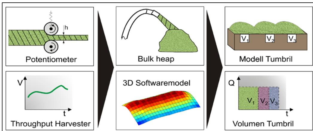
Figure 3: Set up of model based overloading
