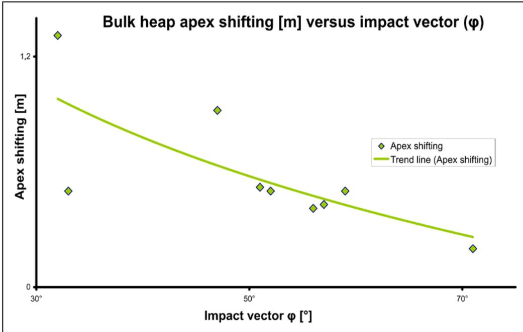
Figure 6: Bulk heap apex shifting versus impact vector
