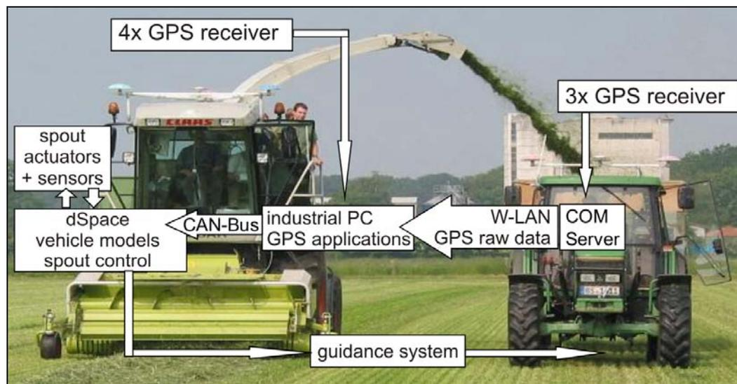
Figure 2: Set up of the ASUL assistance system
