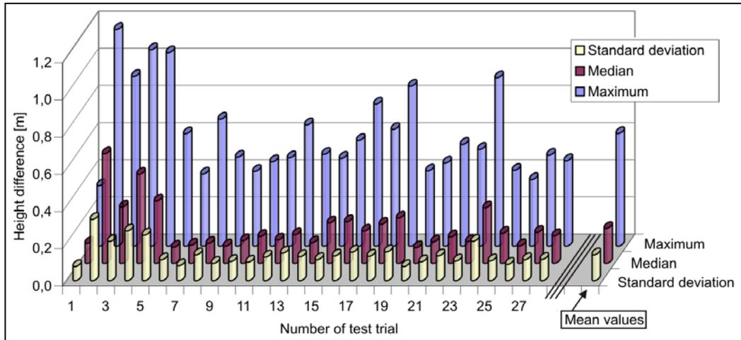
**Figure 10: Maximum, median and standard deviation of the compared height difference**
