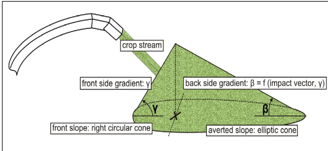
Figure 7: Geometrical bulk heap definition using a bipartite right cone
