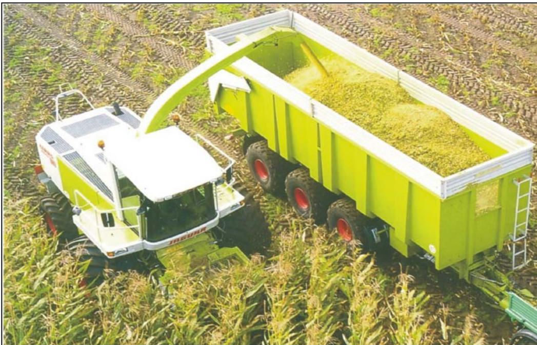
**Figure 1: Self propelled forage harvester and tractor-transport unit**
