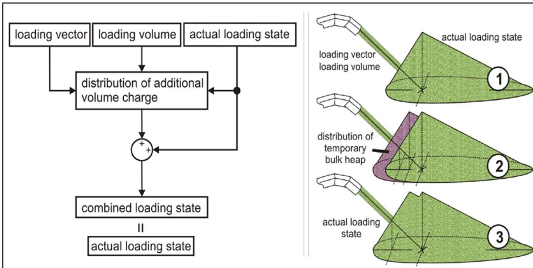
**Figure 8: Software concept of the loading state definition**
