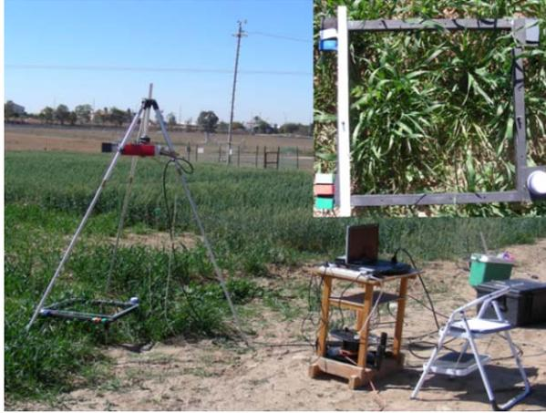
**Fig. 1. Spectral Camera HS in a wheat field, focusing on the sensor point of view – in the frame: wheat, GW and BLW.**
