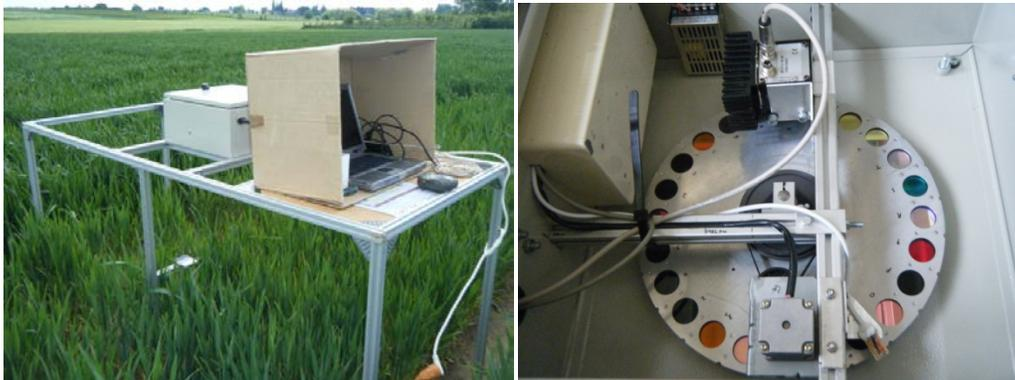
Fig 1. Multispectral vision system (left), table structure with computer, camera and wheel filter (right).
