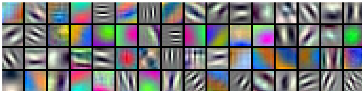
Fig 3. Feature extractor in the first layers of CNN-F model. This filters can detect edges and colors in small areas of an image.
