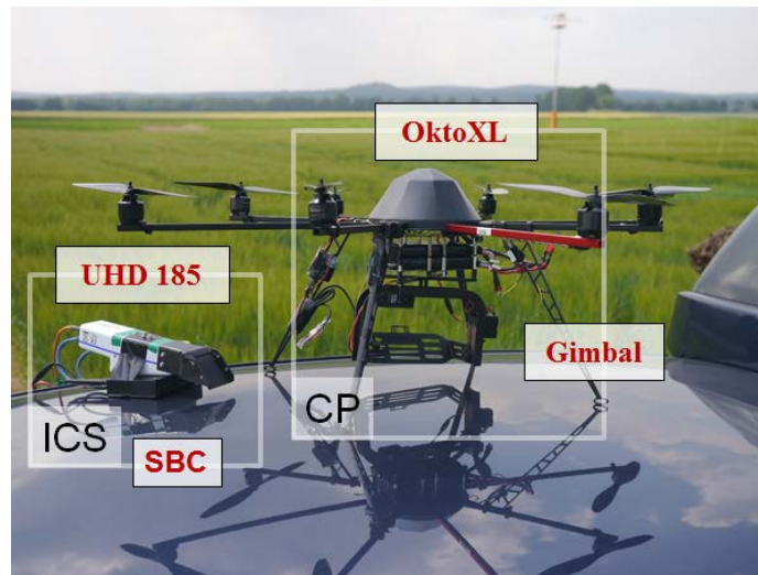
Figure 3 Carrier Platform (CP) MikroCopter Okto XL with Gimbal and image capturing system (ICS) with UHD 185-Firefly and the single board computer (SBC) Pokini Z (Aasen et al., 2015).
