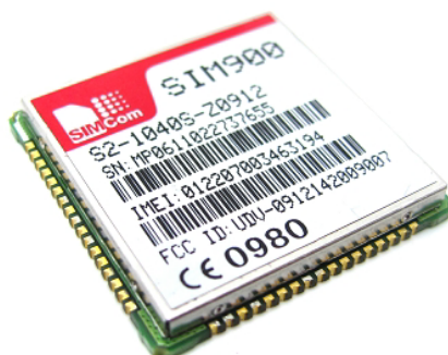
Figure 8. SIM900 GSM module
