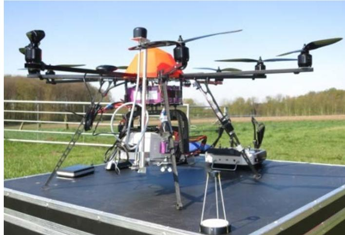
Figure 3: Lightweight crop sensor prototype mounted on MK-Oktokopter UAV-platform.
