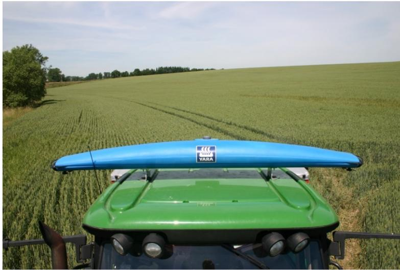
Figure 2: Sensor mounted on tractor-platform.
