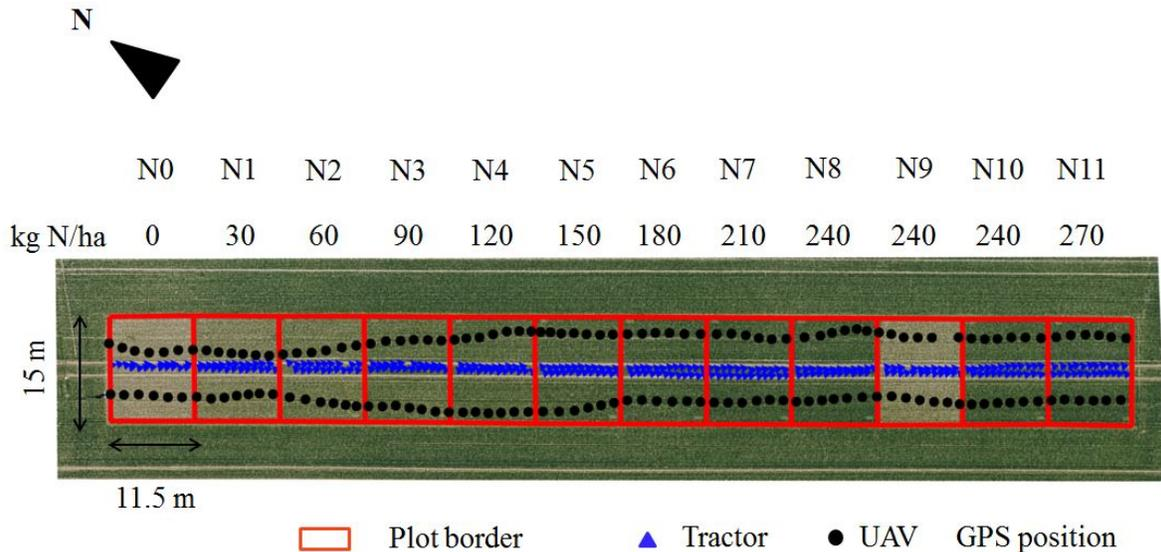
Fig 5. GPS positions for the spectral readings from both platforms.
