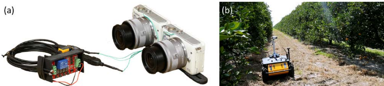
Fig 1. The imaging sensor (5-band camera); (a) two converted Canon M10 mirrorless cameras mounted on a bracket and the shutter controller; (b) the 5-band imaging system mounted on a field robot for autonomous field inspection.
