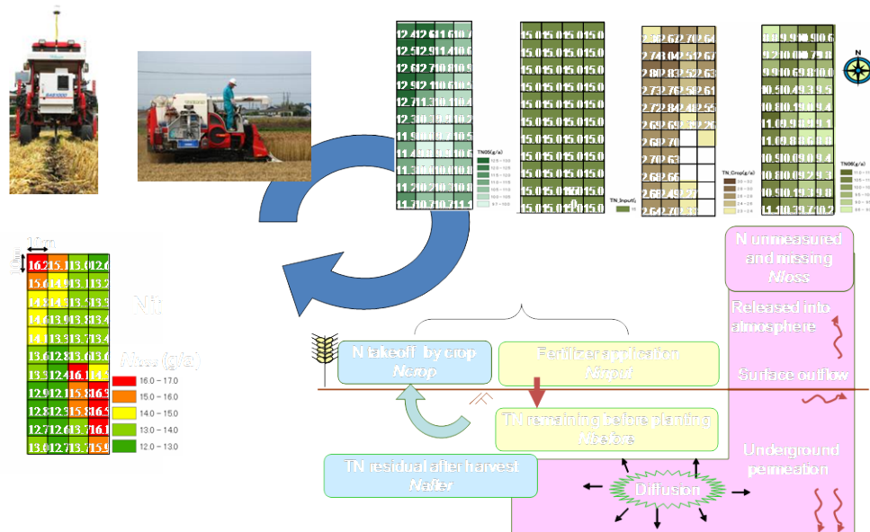
Figure 5. Combination of real-time soil sensor and combine harvester with yield monitor creates missing nitrogen map.
